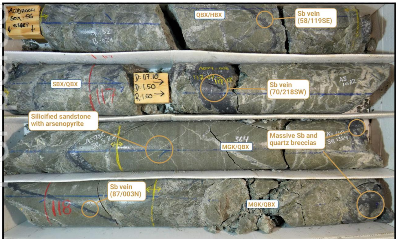
Figure 7a. Fraternal Shoot intersected in AXDDH004 116.2m – 118.5m (SBX - stibnite cemented breccia, QBX – quartz breccia, HBX – host rock breccia, MGK – silicified disseminated arsenopyrite mineralised greywacke, MAR - silicified disseminated arsenopyrite mineralised argillite).
