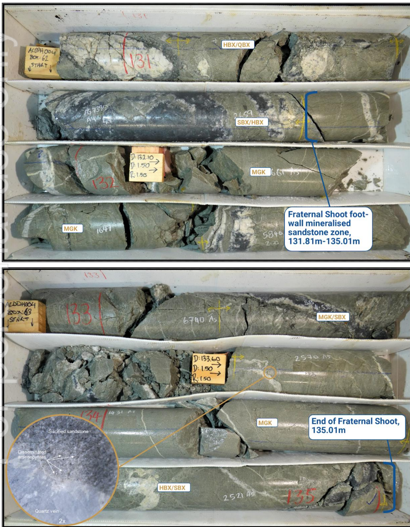
Figure 7e. Fraternal Shoot intersected in AXDDH004 130.9m – 135.0m. Inset photo = acicular arsenopyrite crystals
