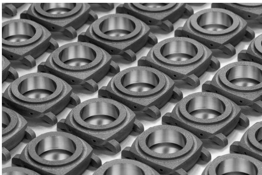
Figure 8: 3D printed watch cases for Officine Panerai, a subsidiary of Compagnie Financière Richemont, using IperionX's low-carbon, 100% recycled titanium powders
