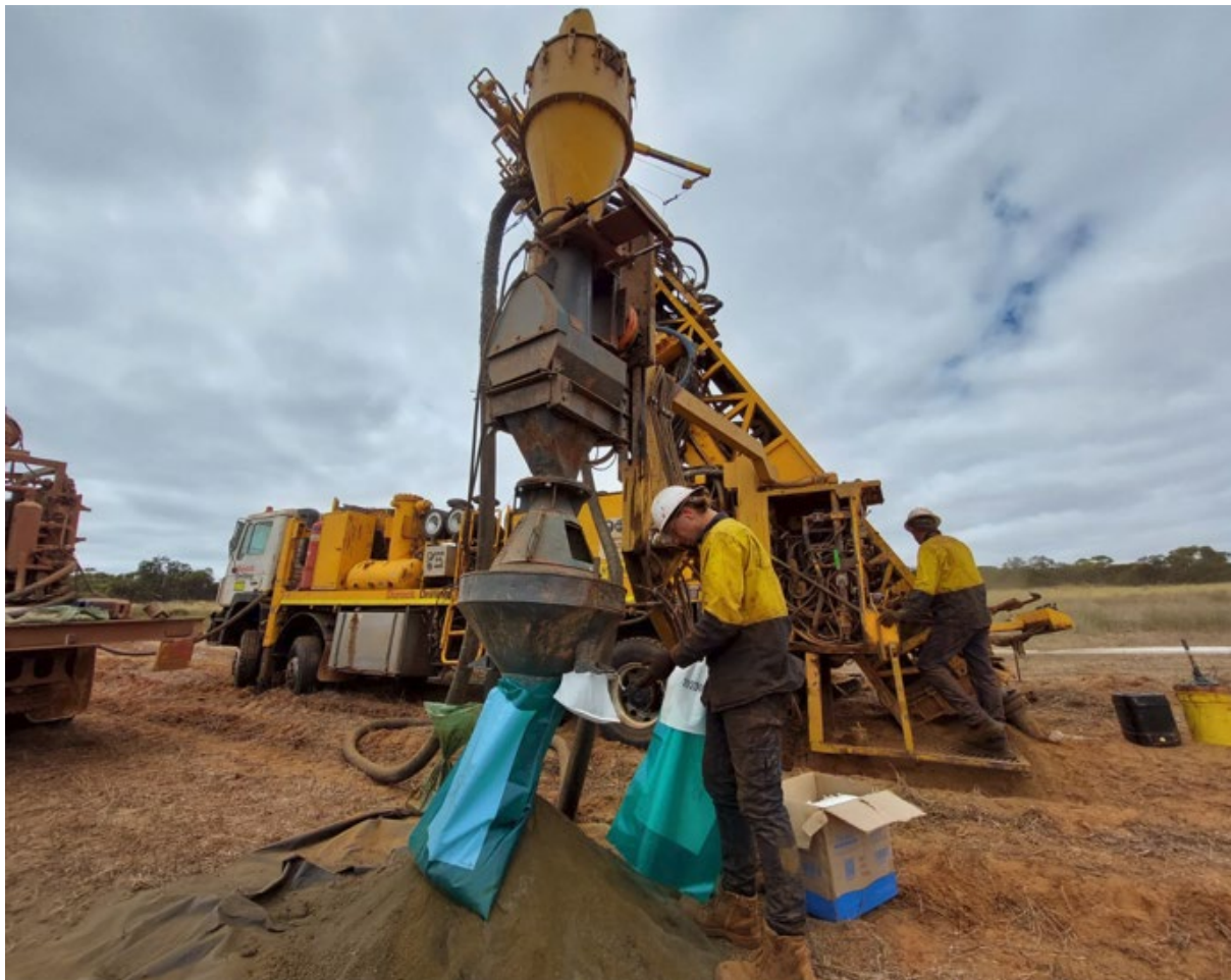
Figure 1: RCP drill rig on location at Jamieson Tank in South Australia
