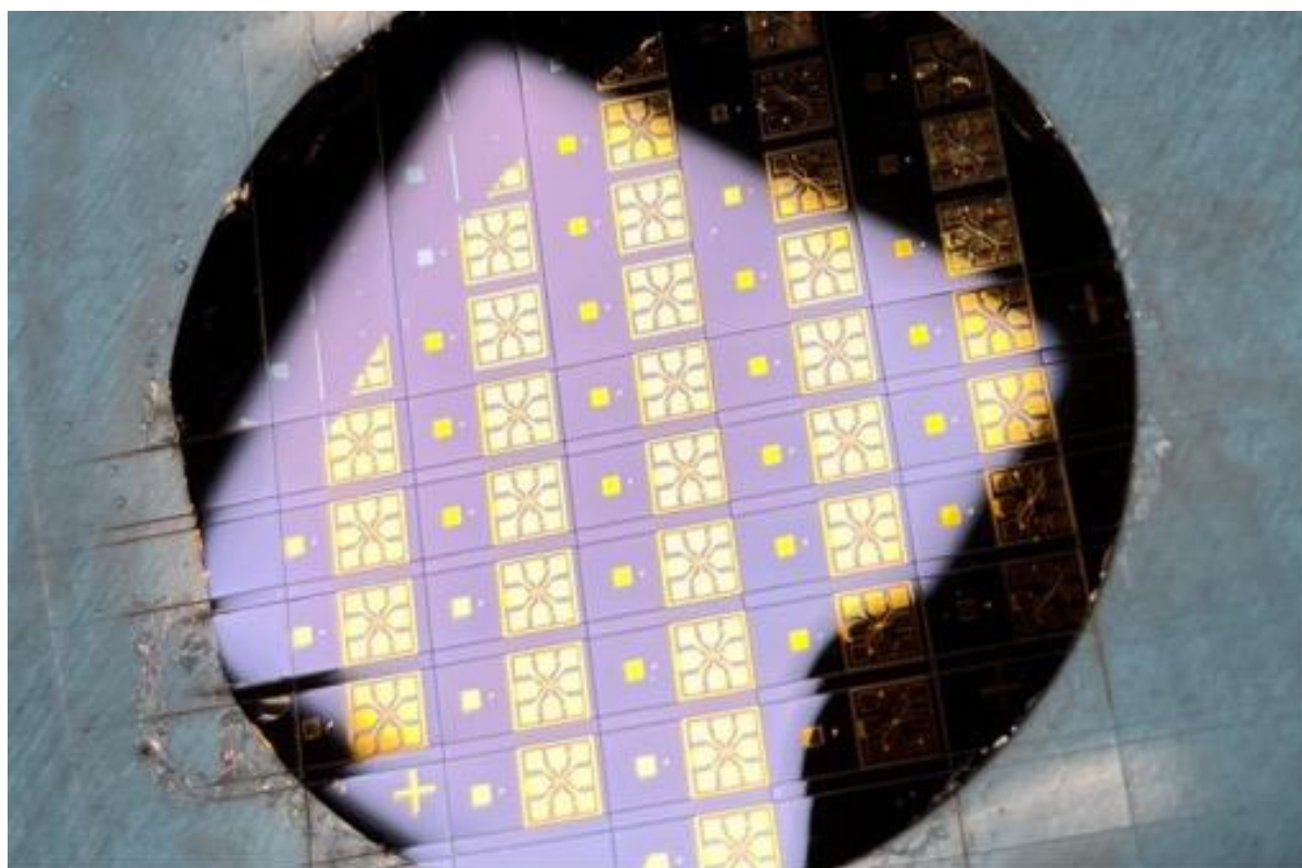
Image 1. A multitude of Archer quantum electronic devices defined by UV optical lithography on a commercial 2" silicon-on-insulator wafer substrate.
