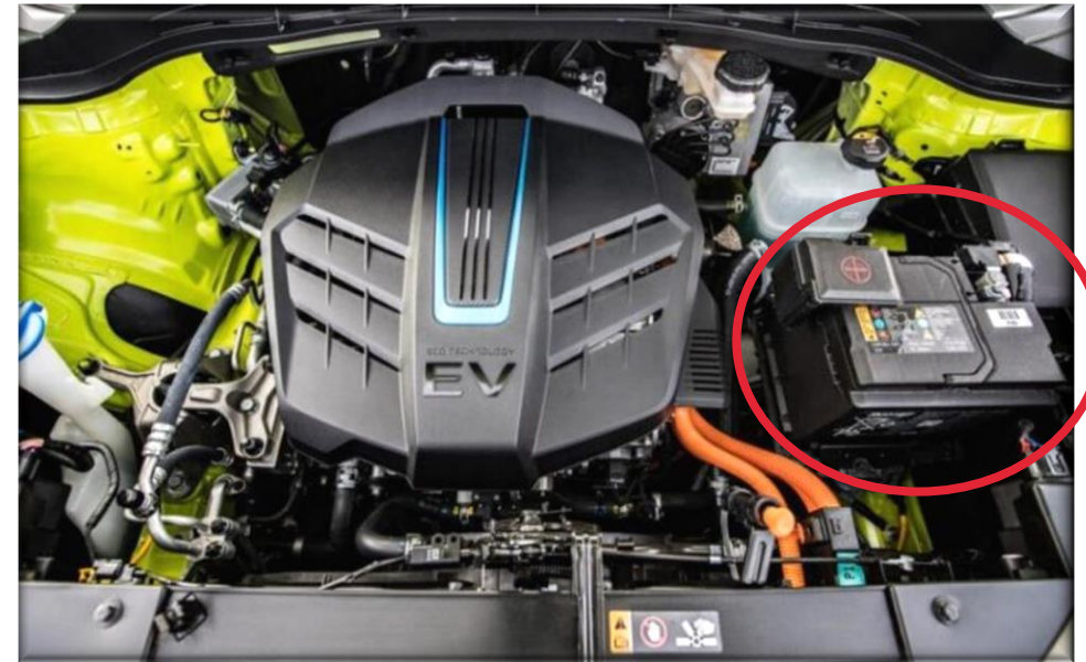
12V lead-acid battery in a Kia Soul EV
