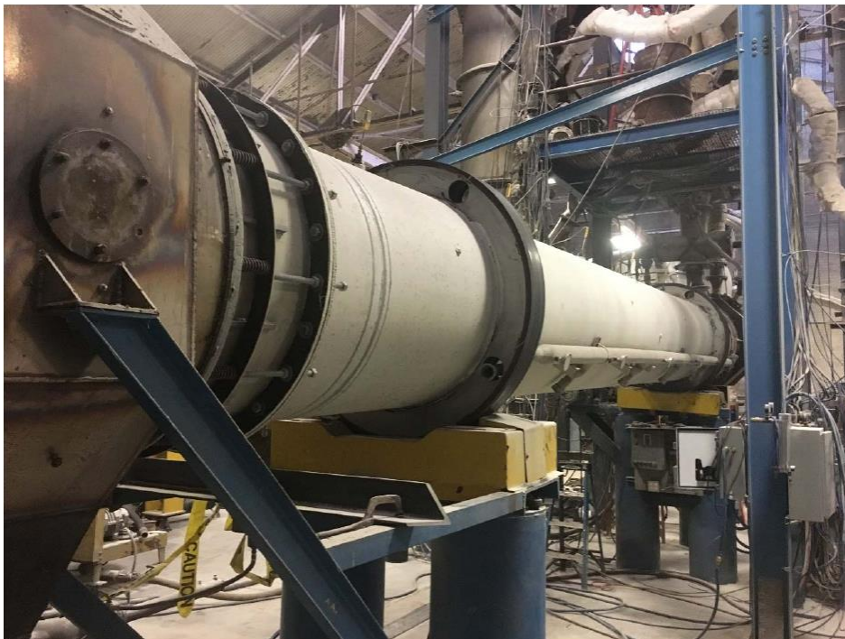
Figure 1: Pilot Rotary Kiln (9.8m long by 0.9m diameter) at FLSmidth Test Facility
