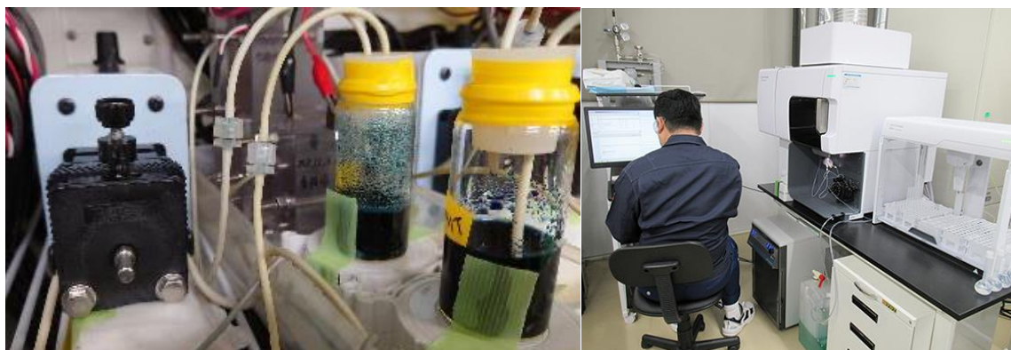
Figure 2: Mini-cell testing of TMT vanadium electrolyte – LE System's Tsukuba Technical Centre, in Ibaraki, Japan. Source: LE System
