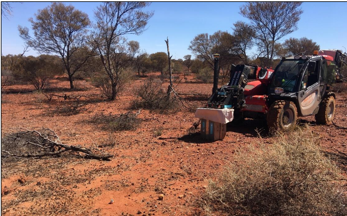
Figure 10. Ultramag eVibe Synchro in the field at Everleigh. The device is small and manoeuvrable, thereby greatly reducing the environmental impact of the survey. The system uses an electrical energy source that eliminates the need for the use of explosives that would have been used for a conventional seismic survey.
