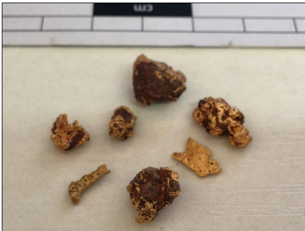
Figure 6. Selection of gold nuggets recovered during this past week in conjunction with rock chip sampling along the Northern Reflector. The nuggets are interpreted to be close to source due to preservation of surface textures and the presence of retained gangue mineral phases.
