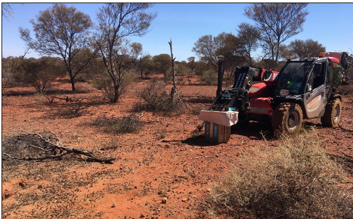
Figure 10. Ultramag eVibe Synchro in the field at Everleigh. The device is small and manoeuvrable, thereby greatly reducing the environmental impact of the survey. The system uses an electrical energy source that eliminates the need for the use of explosives that would have been used for a conventional seismic survey.
