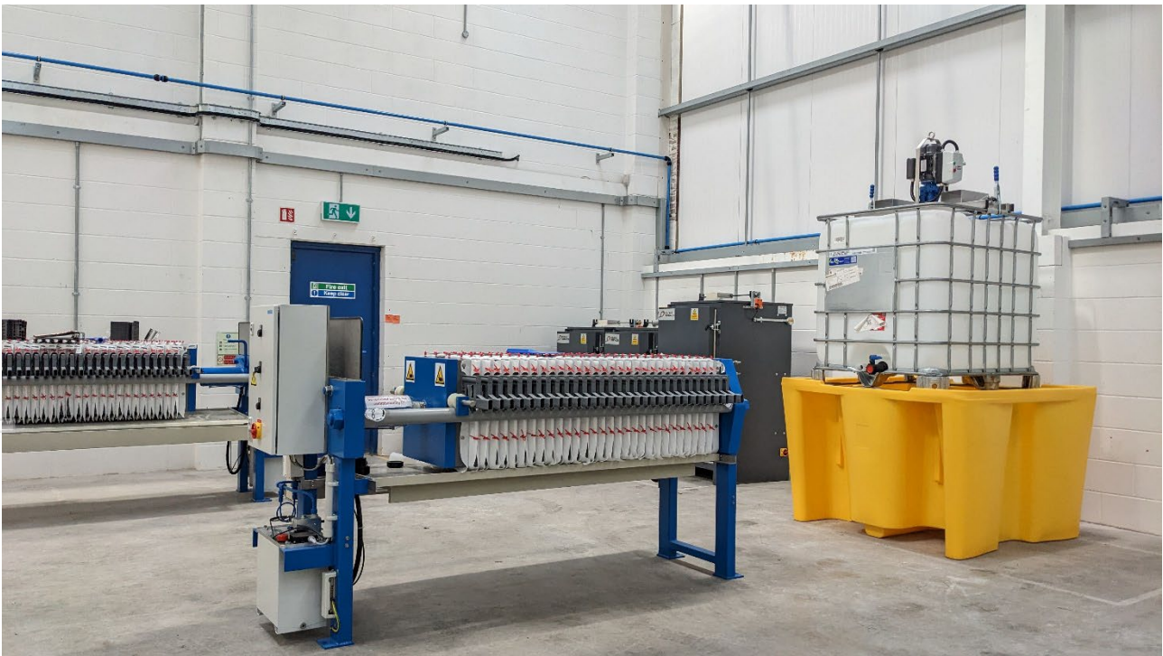
Figure 3: Plate and Frame filters in position along with process vessels and product drying kilns.
