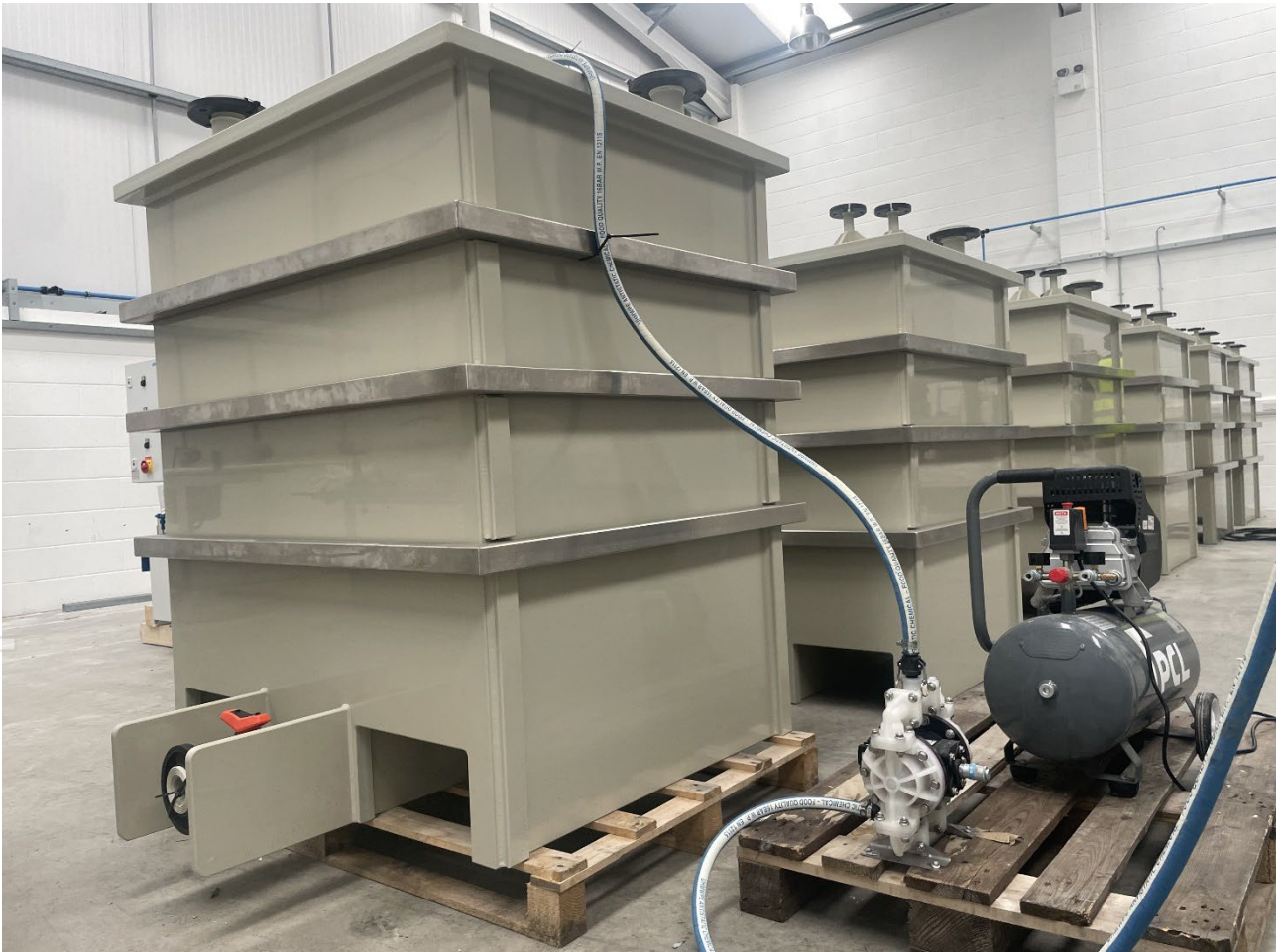
Figure 1: Process reactors undergoing hydrostatic testing.
