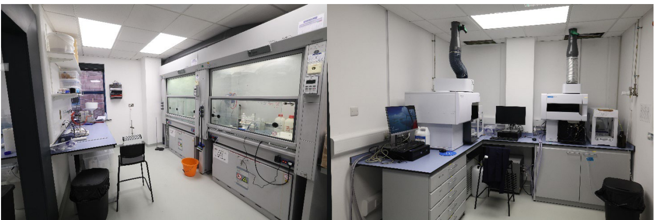
Figure 10: Hydrometallurgical and analytical wet labs now operational, supported by two Inductively Coupled Plasma Optical Emission Spectroscopy (ICP-OES) instruments.
