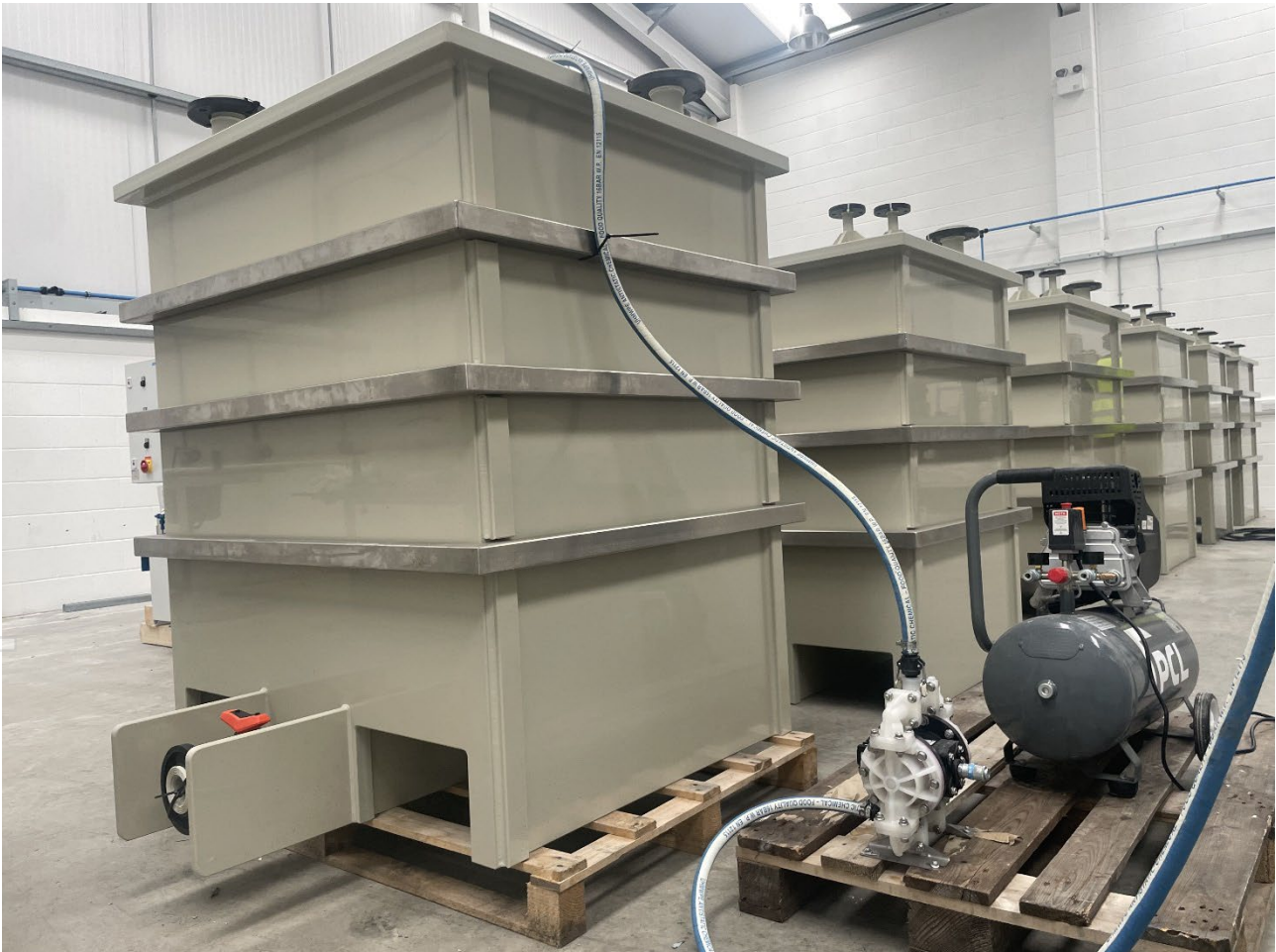
Figure 1: Process reactors undergoing hydrostatic testing.
