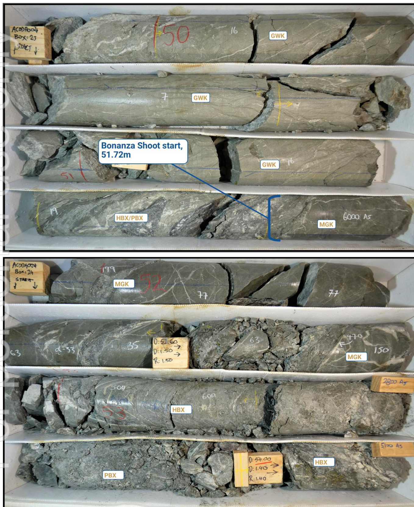
Figure 8a. Bonanza Shoot intersected in AXDDH004 51.7m – 54.2m (QBX – quartz breccia, HBX – host rock breccia, PBX – pug breccia, MGK – silicified disseminated arsenopyrite mineralised greywacke and FLT - fault).
