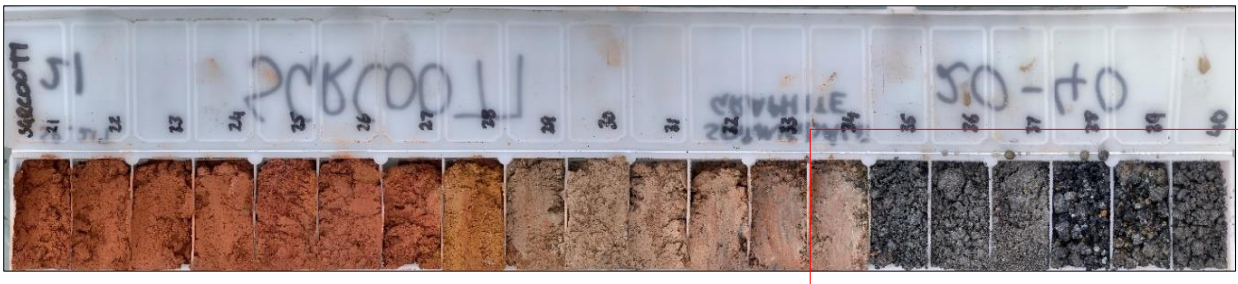
Figure 3: RC chips from SGRC0077, 33-42m, 9m @ 17.27%, including 4m @ 29.33%
