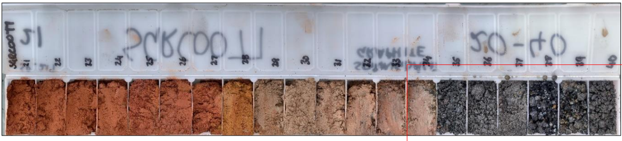
Figure 3: RC chips from SGRC0077, 33-42m, 9m @ 17.27%, including 4m @ 29.33%
