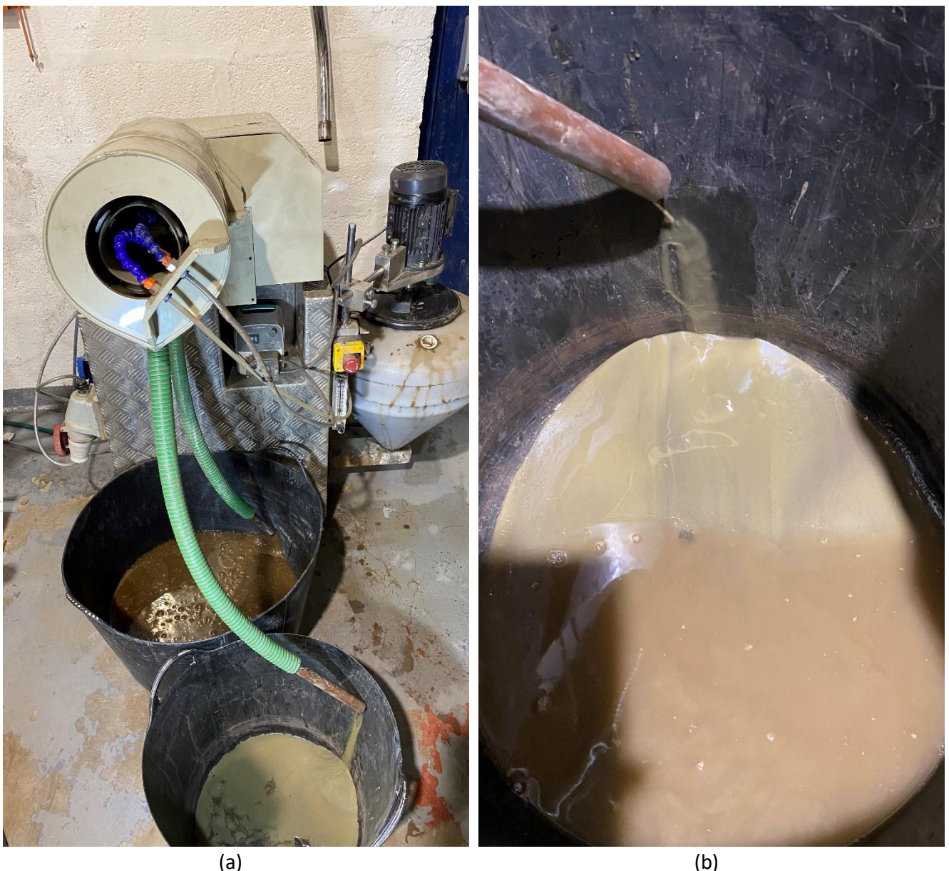
Figure 3. (a) Testing using the Micro MGS at Gravity Mining in the UK. (b) REO concentrate product from the MGS.
