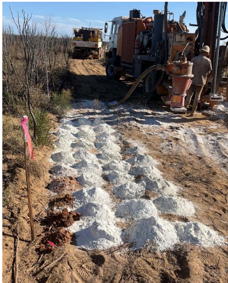
Figure 1. High quality Kaolin intersected 30m of bright white kaolin from 4m depth (KAC014).
