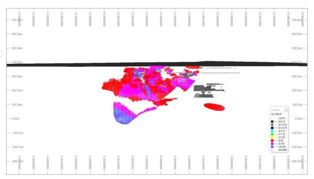
Figure 13: Long section showing underground working and topography (grey) with domains 1, 2 and 3 indicated and inferred resource with Au>2.5g/t. Model displayed with AU\_cut.
