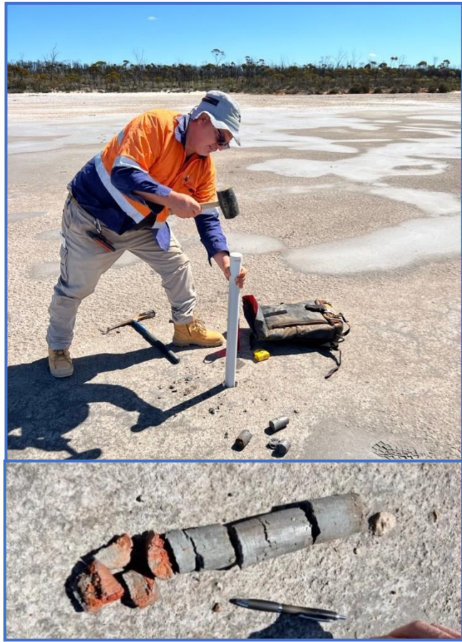
Figure 2. Lake Hope showing the push tube sampling method (!) and an example of the lake clay from the push tube.
