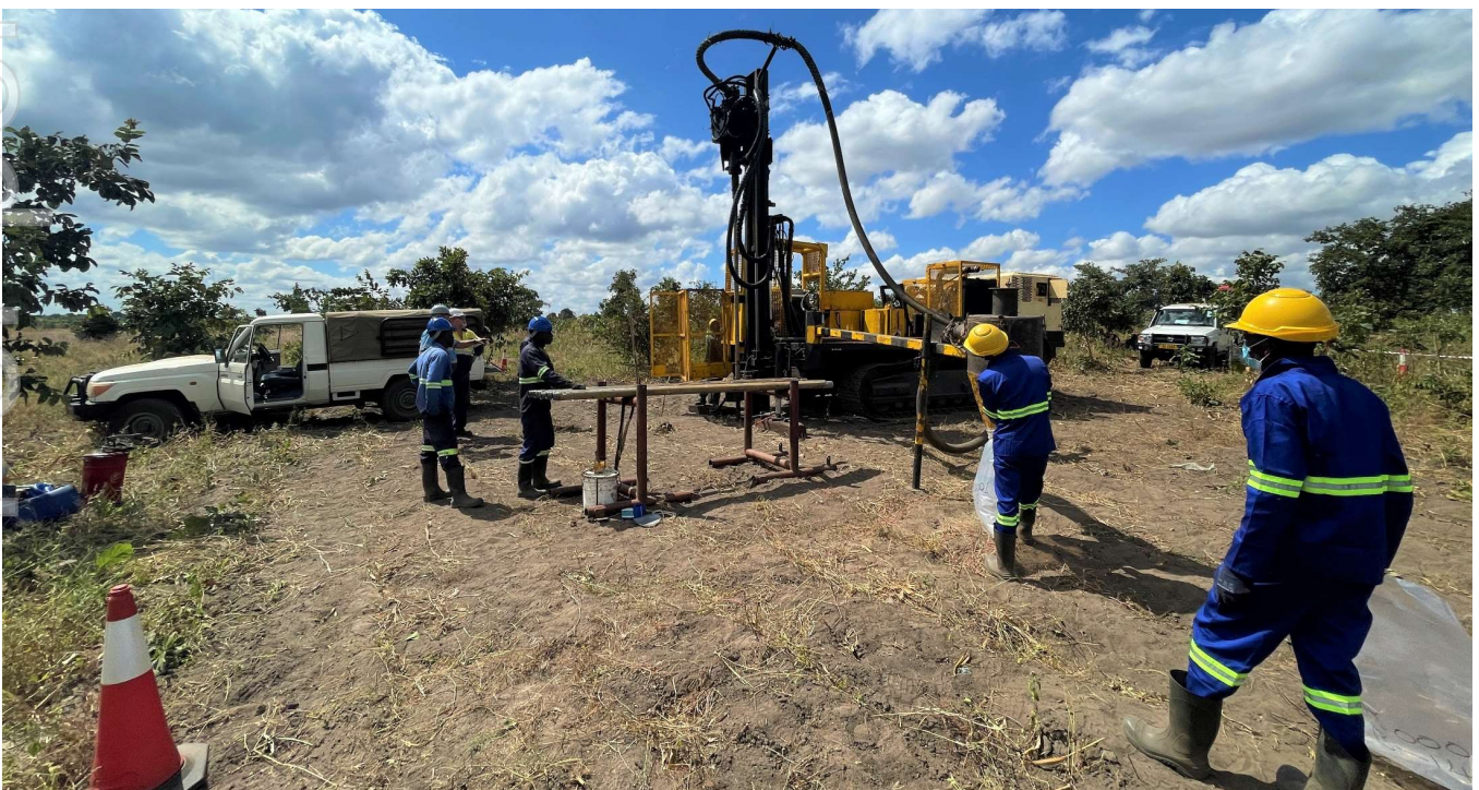
Figure 8: Air-core (AC) drilling at Kasiya in May 2022.
