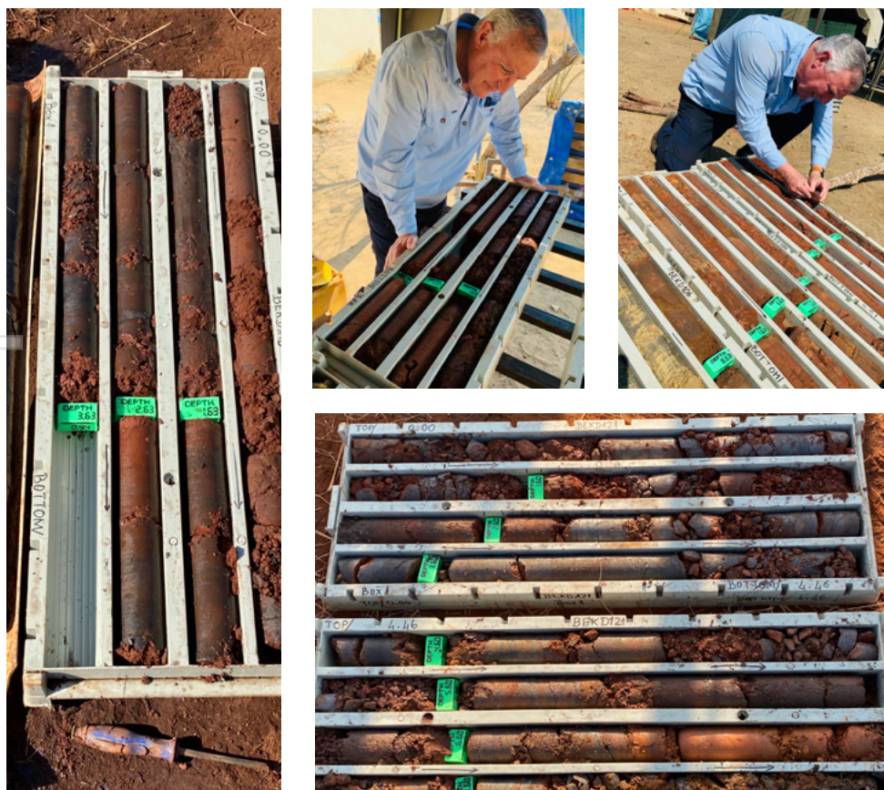
Figure 9: Drill core from the in-fill drilling showing high-grade iron mineralisation as determined by magnetic susceptibility reading of >1000, these drill intercepts appear to be between ~10 metres to ~14 metres thick.
