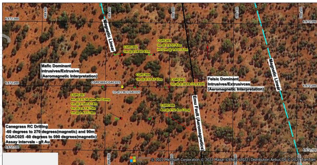
Figure 7: RC Drill Collars with significant gold intersections
