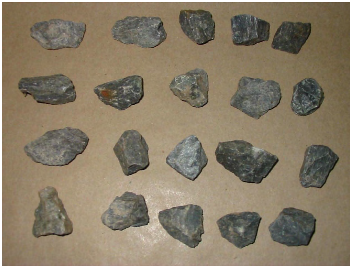
Figure 4 – A Typical Set of Particles for Breakage (Particle Selection Method)
