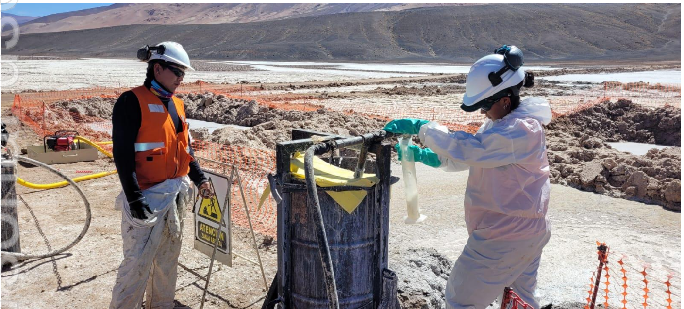
Figure 1: Brine sampling from drillhole PM23-IN-03 at the Incahuasi salar, Salta Lithium Project.
