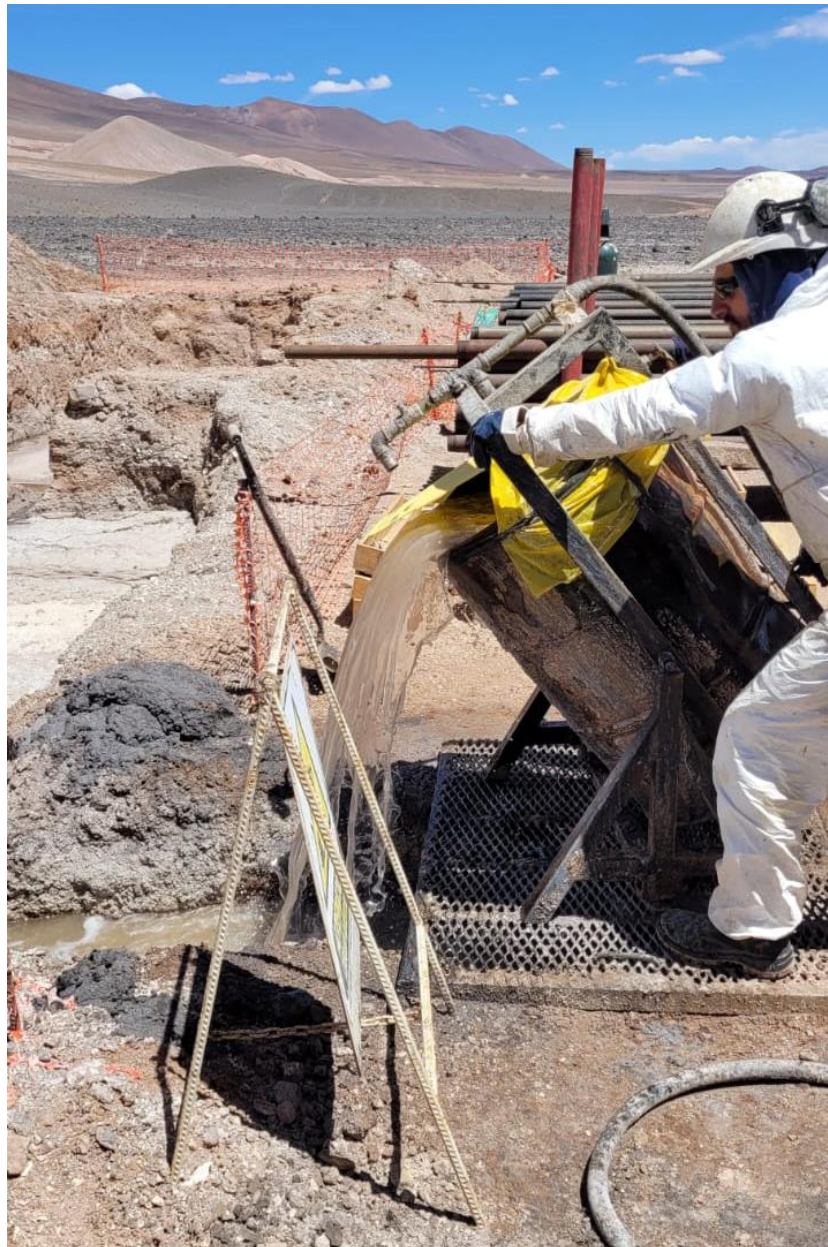
Figure 2: Brine sampling from drillhole PM23-IN-03 at the Incahuasi salar, Salta Lithium Project.
