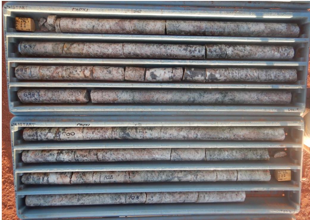
Figure 5 – MAD213 from 696.10m to 703.4m showing a portion of the 120m+ intersect of coarse-grained pegmatite from the Manta seismic reflector
