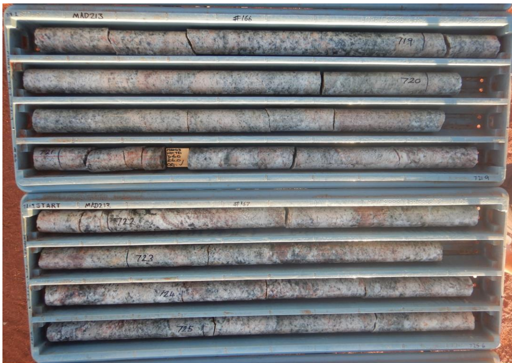
Figure 6 – MAD213 from 718.2m to 725.6m showing a portion of the 120m+ intersect of coarse-grained pegmatite from the Manta seismic reflector
