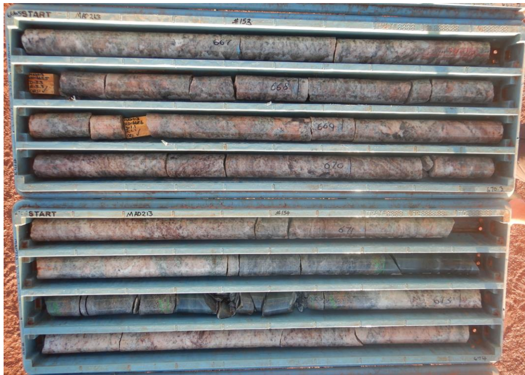
Figure 4 – MAD213 from 666.50m to 674m showing a portion of the 120m+ intersect of coarse-grained pegmatite from the Manta seismic reflector
