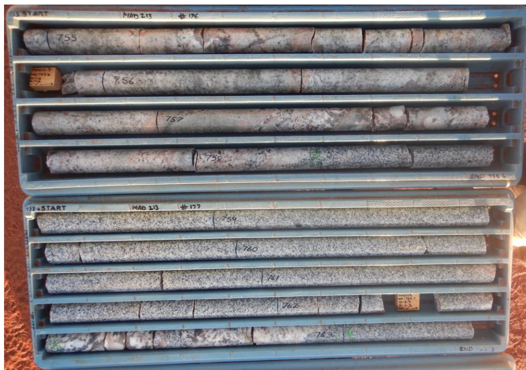
Figure 8 – MAD213 from 755m to 763.3m showing a portion of the 120m+ intersect of coarse-grained pegmatite from the Manta seismic reflector in contact with footwall granite at 758.2m
