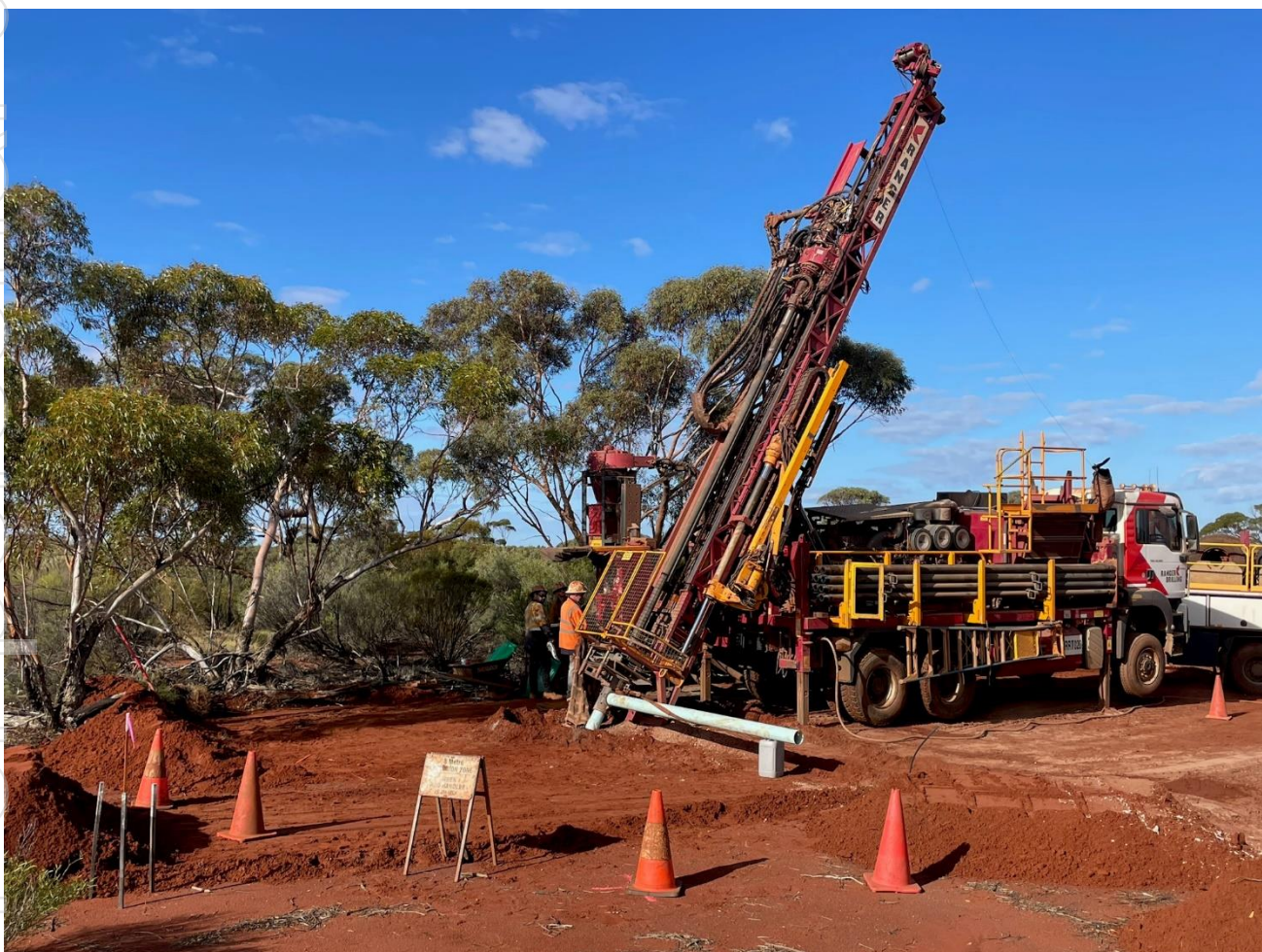
Figure 1 RC Rig set up on first hole of Comet Vale program
