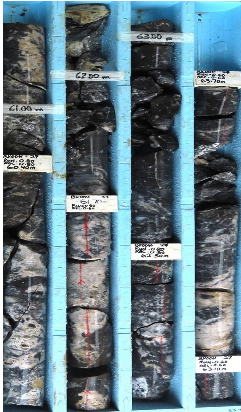
Figure 2: Portion of BKDDH-27 core, between 60.0m-63.7m, illustrating intense alteration in a zone hosting bonanza gold grades: 0.5m @ 209 g/t between 60.5m – 61.0m; 1m @ 64 g/t between 61.0 – 62.0 m; 1 m @ 15.9 g/t between 62.0m – 63.0m & 1m @ 31.8 g/t between 63.0m – 64.0m.
