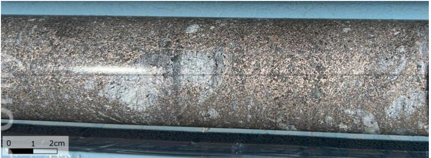
Fig2: Photo of core from BUDD0001 showing the first sulphidic conductor returning 1.13m at 1.83g/t Ag and 0.12% Cu from 46.39m
