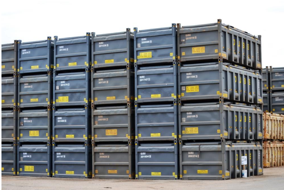
Figure 2 –Lead-silver concentrate containers at the Geraldton Port waiting transport for ship loading (Photo 24 March 2023).
