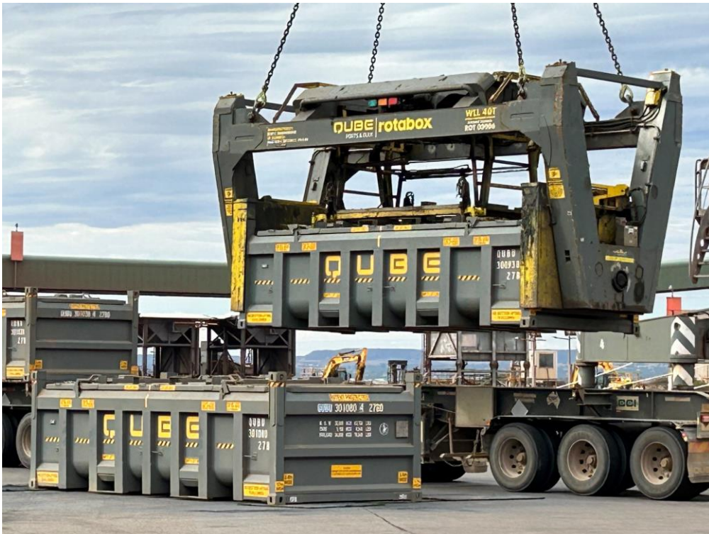
Figure 4 – Closeup view of the Rotabox system at work with the lifting and transfer of concentrate to the ship hold. Once inside the ship hold, the lifting mechanism rotates the container to place the concentrate in the hold (Photo 24 March 2023).
