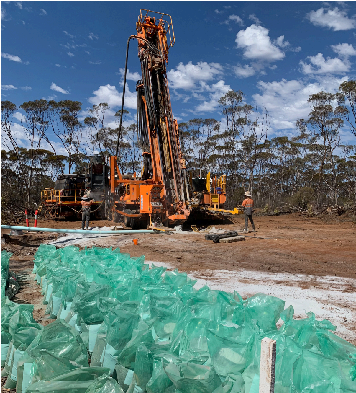
Photo 1 Reverse circulation drilling at Darson South – March 2023.
