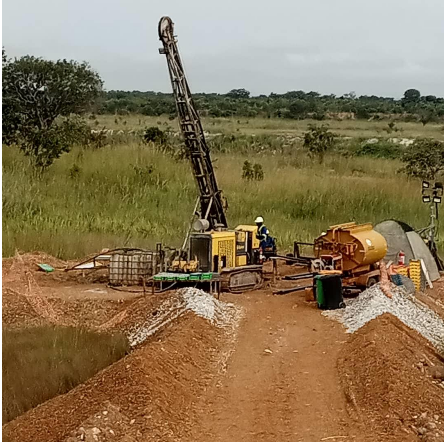
Figure 7: Drilling on causeway built over marshy ground. Roche Dure pit in background
