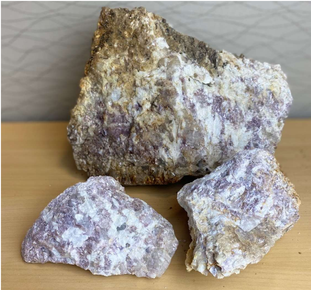
Photo (A): Rock samples from Pink Panther (Kanchanaburi) where LIBS analyser testing confirmed 3.45% Li (7.4% Li 2 O) in lepidolite (pink minerals) bearing pegmatites
