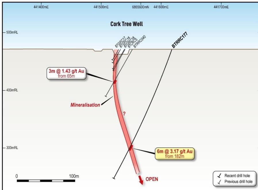
Figure 7: Cross Section of CTW with BTRRC177.
