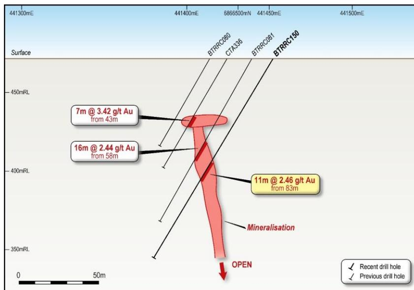
Figure 5: Cross Section of Orebody 4 with intersections.
