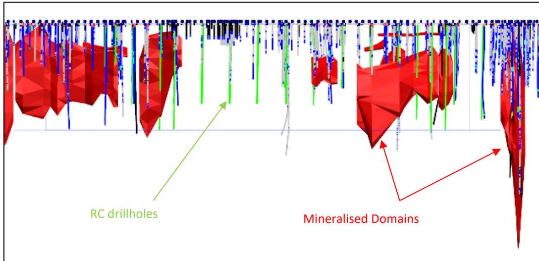
Figure 4: Long Section of RC drill program hole locations (north of pits).
