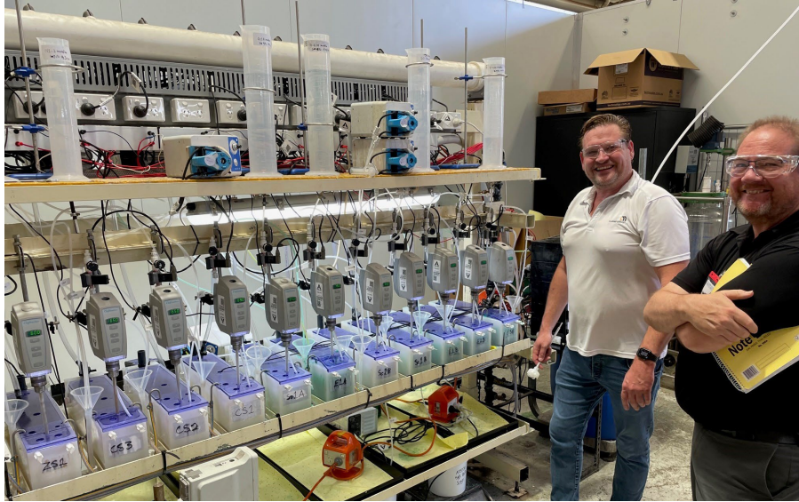
Figure 5: Phase 2 Pilot - Zinc & Calcium Solvent Extraction (with Principal Metallurgist, John Knoblauch and GM Operations, Wayne Foote)
