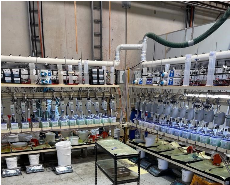
Figure 6: Phase 3 Pilot - Cobalt and Manganese Solvent Extraction & Nickel Purification
