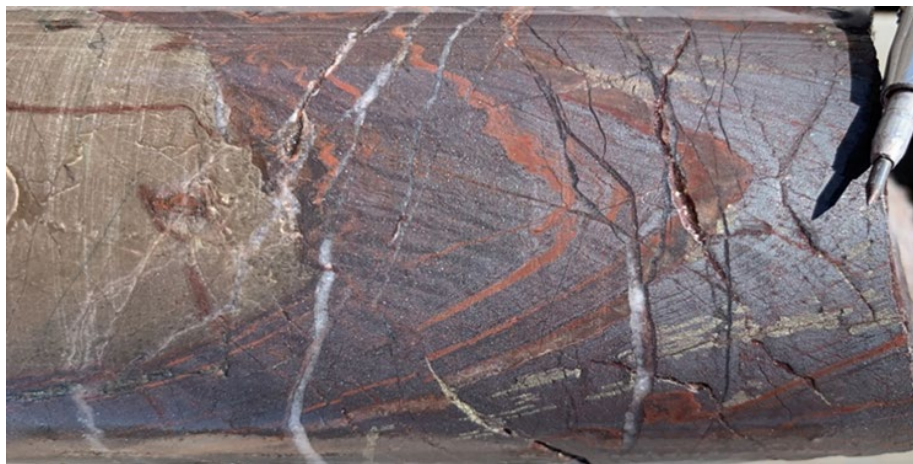
Figure 5. Hematitic ironstone and pyrite (sulfide mineral) mineralisation (482.3m).
