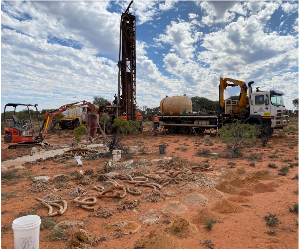
Figure 11. Water Well rig drilling at LWP002.
