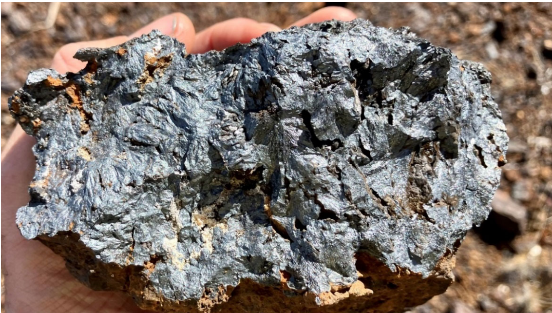
Figure 9. Manganite sample showing pyrolusite needles (Sample#ZEU110).
