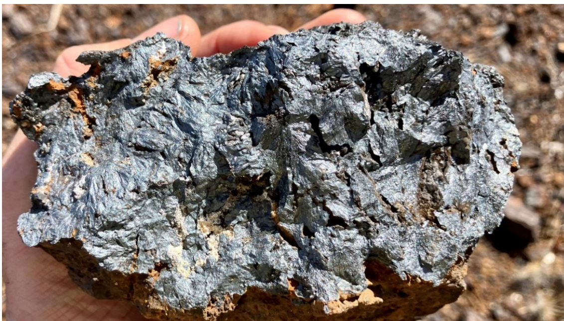
Figure 9. Manganite sample showing pyrolusite needles (Sample#ZEU110).
