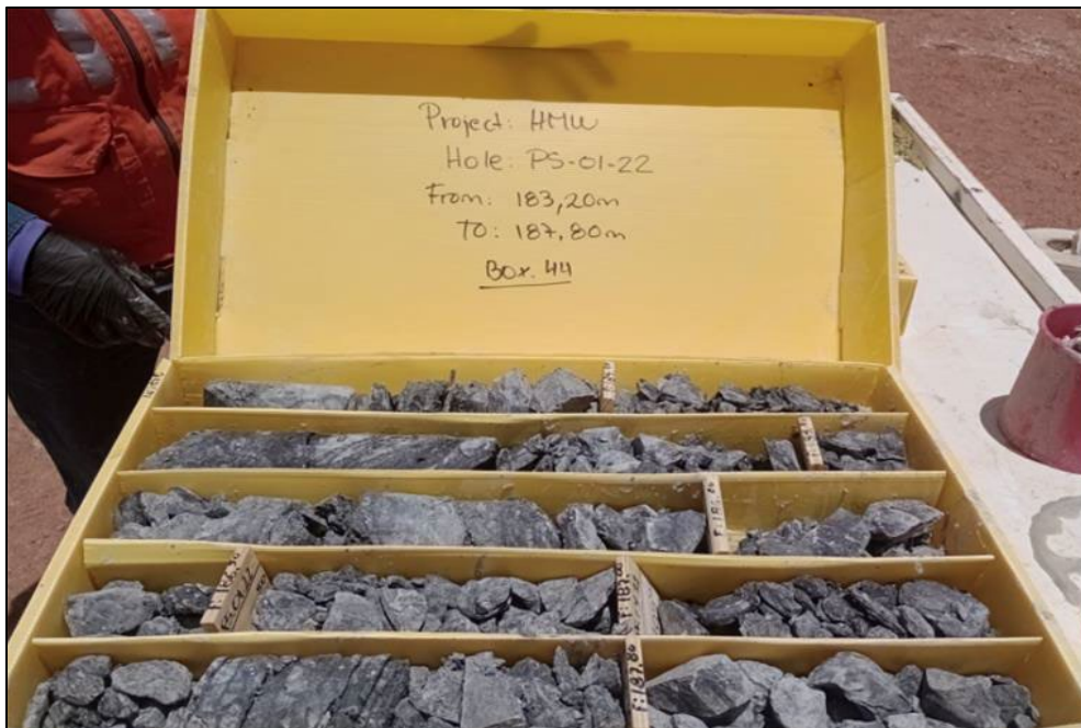
Figure 7 - Highly fractured rock core obtained from PS-01-22
