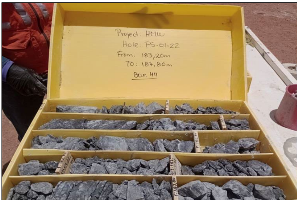
Figure 7 - Highly fractured rock core obtained from PS-01-22
