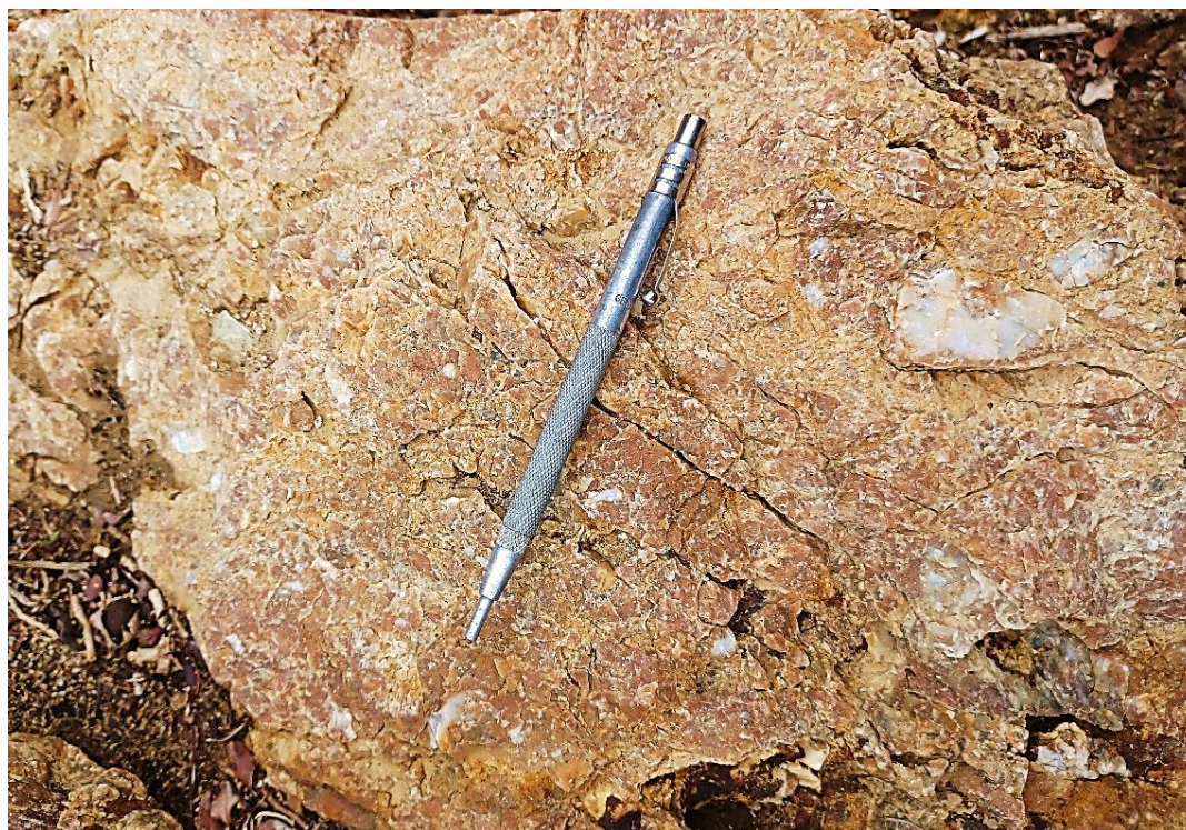
Figure 8: Silicified breccias identified at the T4 target area (refer ASX announcement 23 August 2022).
