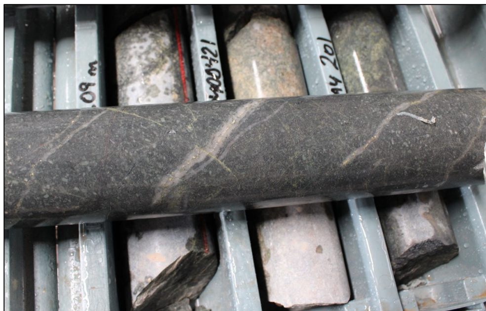
Figure 4. HQ diamond core from Corvette diamond hole 22MYDD421 at 817.5 metres, highlighting the abundance of early quartz veins with a centre-line of sulphides (also known as B-veins) crosscut by later epidote-chalcopyrite veins. This mineralisation forms part of a zone that grades 13 metres at 1.07% Cu & 0.61g/t Au (ASX MAG 30 January 2023).
