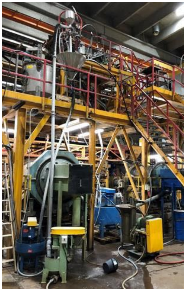
Figure 4.1.1: Pilot Plant: Grinding Circuit with Ball Mill (bottom left), Screening (top middle), and HydroCyclones for Desliming (top left)
