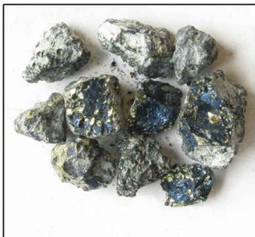
Photo 7. Lode-style copper mineralisation from TGAC078, very similar to the Cayley Lode mineralisation – proximal to the Junction 1 soil copper anomaly. Massive- to semi-massive pyrite-chalcopyrite with secondary chalcocite-covellite fracture coatings.
