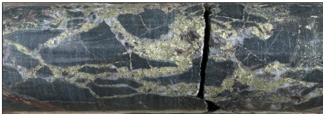
Photo 5. Chalcopyrite-quartz-hematite fill jigsaw breccia in chlorite-silica altered microdiorite - SMD173, 390.6m drill depth, HQ diameter uncut drill core. Note the dominance of chalcopyrite and hematite and the almost total lack of pyrite as distinct from the previous samples in SMD032, SMD044W1 and SMD050.
