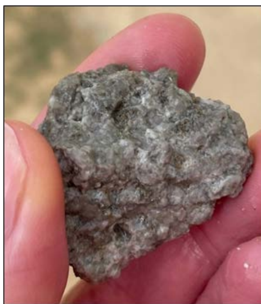
Photo 8. STAC0071 - Silica-sericite-pyrite (phyllitic) altered dacite porphyry at 81m.
