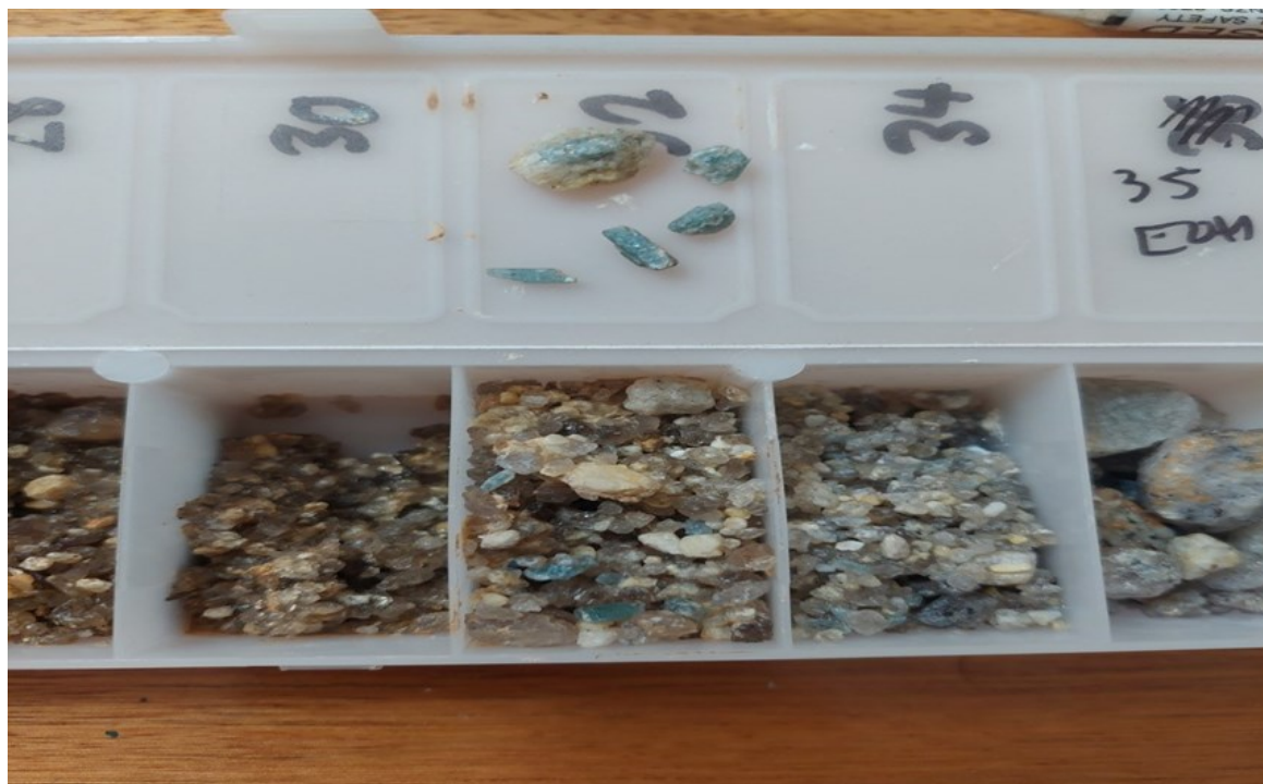
Figure 4. Chip tray showing the final 5m (30-35m) of hole 22DAC016. Downhole meterage is shown. The distinctive blue-green mineral is illustrated amongst the pegmatite chips.
