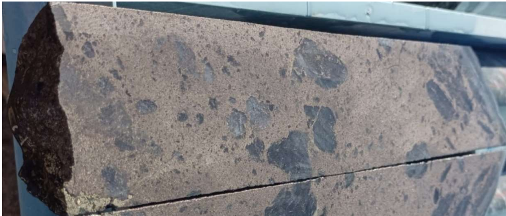
Image 1: Massive/breccia sulphides in SBDD005 at 381m downhole, split HQ core.
