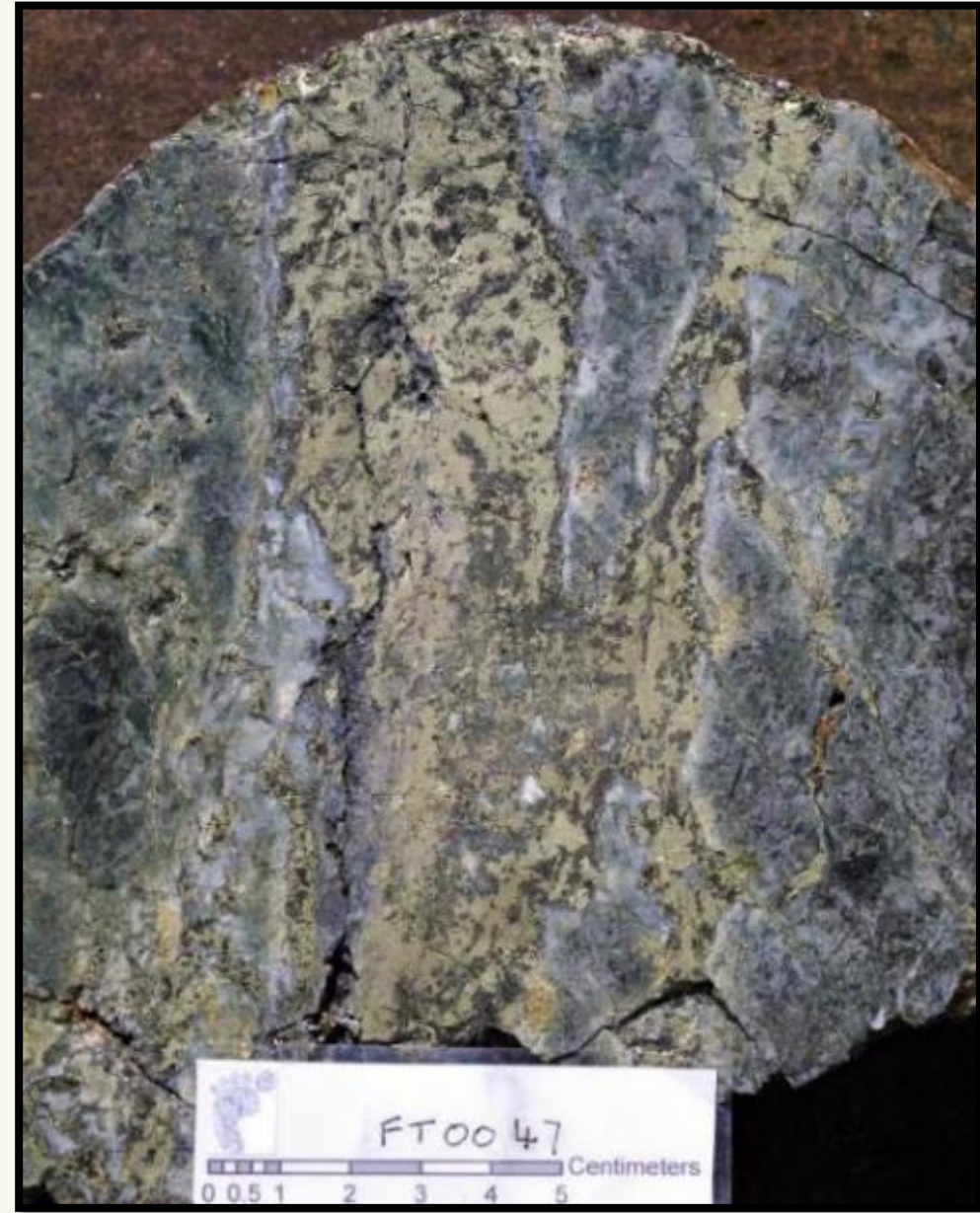
Copper/gold polished sample from Ubei Target. Chalcopyrite-silica-arsenopyrite-pyrite. 9.5% Cu, 156g/t Au Sample 0047. See ASX Release 25.11.22. The Company confirms that it is not aware of new information that affects the information contained in the original announcement.
