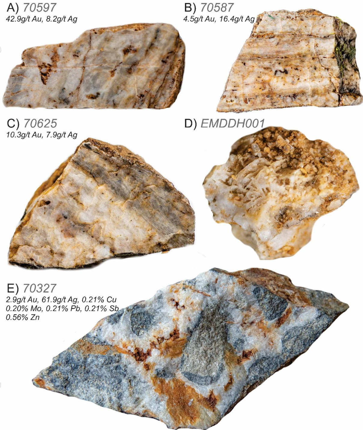
Figure 2 – Examples of epithermal vein mineralisation styles from the Crawley's Reef and Sulphide Shaft area. A) Crustiform banding in sample 70597 (Crawley's Line). B) Laminated quartz-sulphide vein with some crustiform banding on margins (sample 70587, Crawley's Line). C) Comb quartz in sample 70625 (Crawley's Line). D) Bladed silica boiling textures in EMDDH001 (Sulphide Shaft). E) Multi-generational cockade breccia from Sulphide Shaft, displaying early pyrite-sphalerite and later tetrahedrite-rich coatings embedded in silica (sample 70327).
