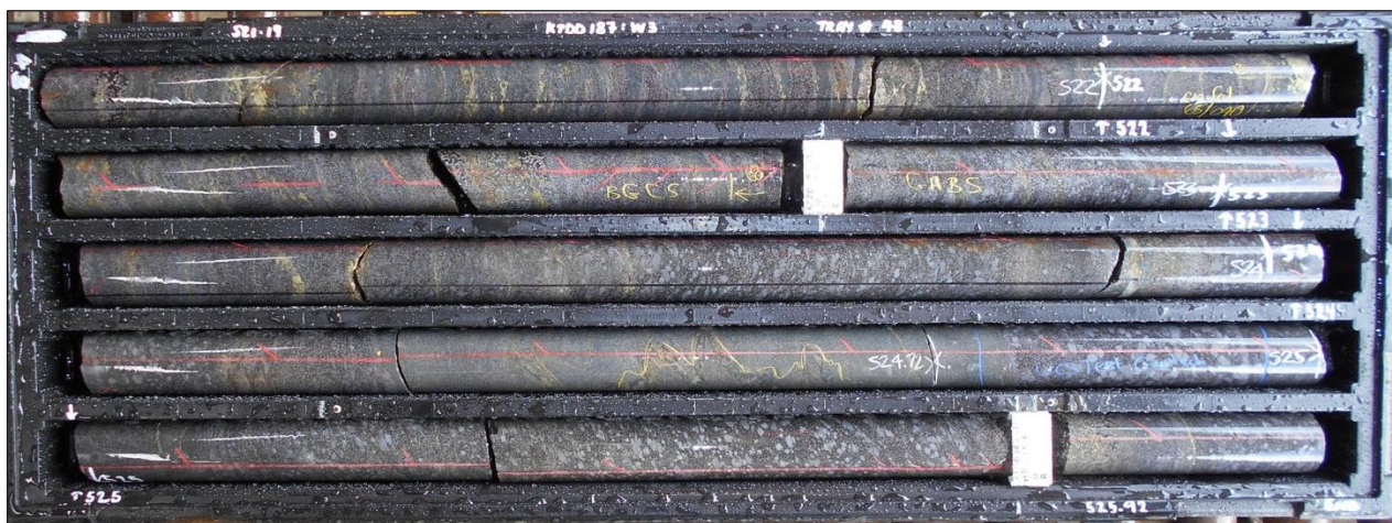
Figure 6: West Kavanagh core (KTDD187_W5 from 521.2m to 525.9m downhole) showing the interbedded GABS and BCGS within the mineralised shoot
