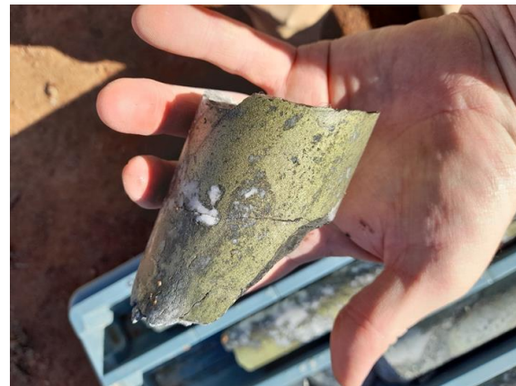
Figure: KSNDDH015 - 71.9m: Chalcopyrite vein. Sample interval 71.6m to 72.3m: 5.5% Cu, 0.5g/t Au, 13g/t Ag.
