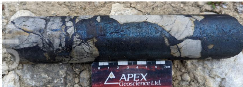
Massive/breccia bornite hosted within dolomite (light grey) in drill hole ST22-05.
