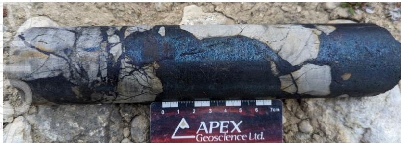
Massive/breccia bornite hosted within dolomite (light grey) in drill hole ST22-05.
