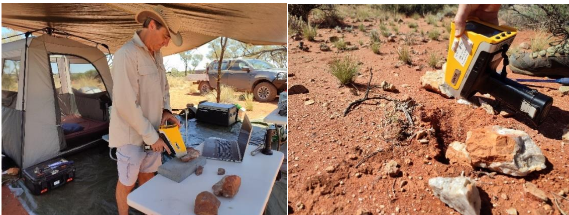
Figure 4 and 5: Portable XRF was utilised to assess individual rock samples and map areas of enhanced prospectivity for follow-up geophysics surveys.
