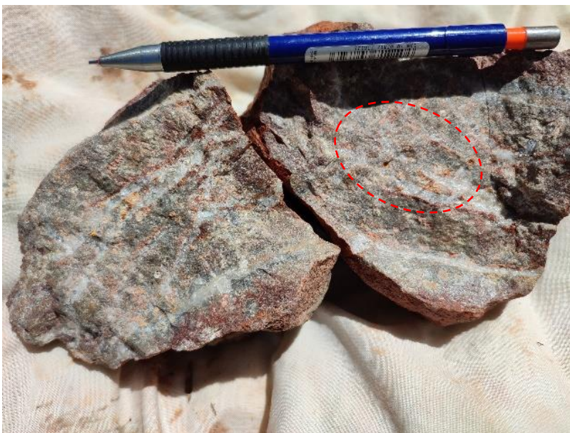
Figure 2: Offset and crosscutting quartz veins indicate development through multiple pulses and support field observations for a large hydrothermal-magmatic porphyry style event at Merino Prospect.
