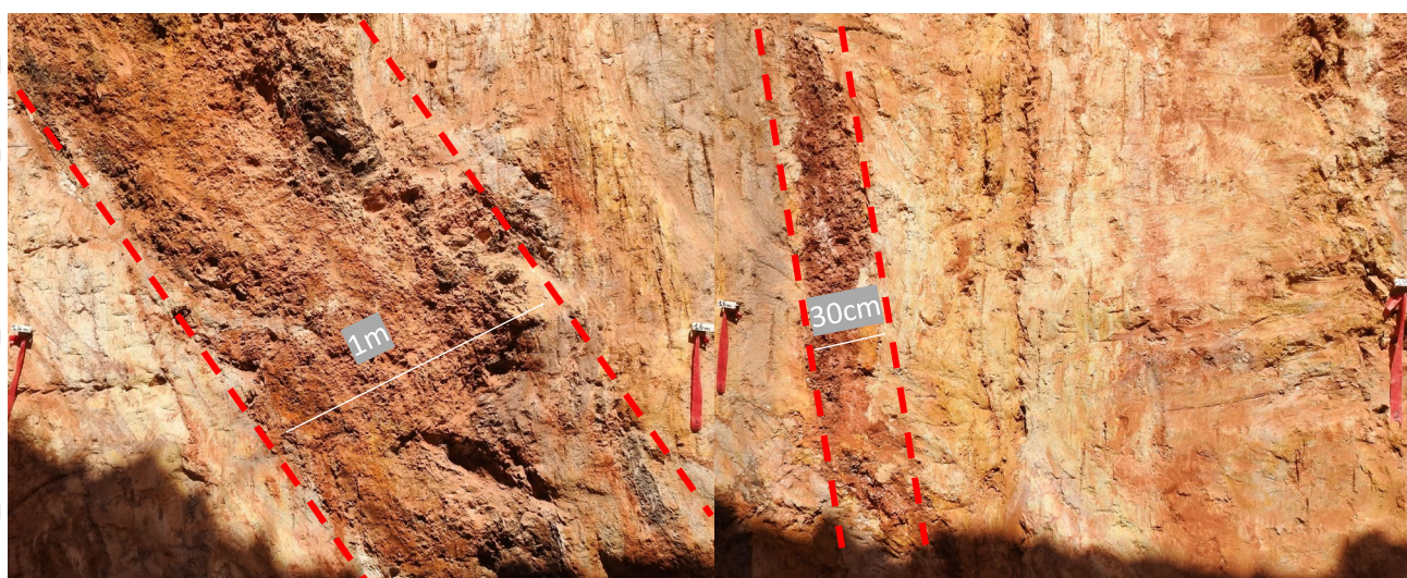
Figure 4: Trench MSTR02 from 14 to 18m, looking north, showing 1m wide moderate east dipping and 30cm sub-vertical mineralised structures. Assays are 2m composites.
