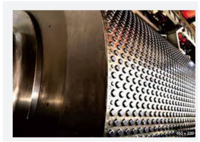
Image of an abrasion resistant HPGR studded roll
