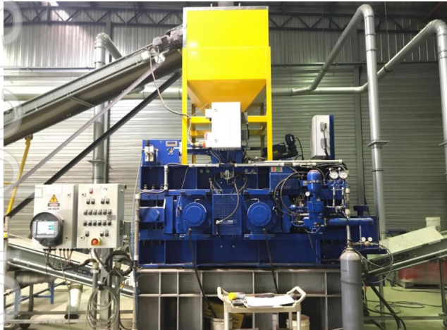
HPGR test unit at Bureau Veritas Minerals Laboratory, Perth, Australia
