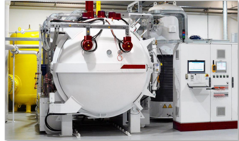
Nadcap Certified Vacuum Braze Furnace – used to braze cold plates. Facility being replicated in the United States to support expansion in the Aerospace and Defence market
