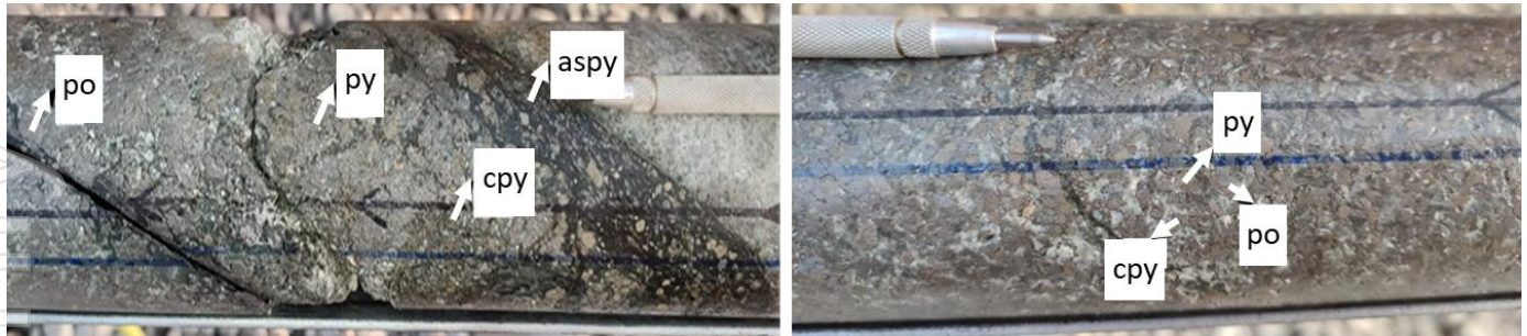
Plate 2. Left: MGDD22-010- First structure (68.9 m) showing the mineralised intercept (31.5g/t gold, 24.3g/t silver and 0.25% copper), it corresponds to massive sulphide vein. Right: MGDD22-010- Second structure (73.15m) showing the mineralised intercept (99.8g/t gold and 89.9g/t silver and 0.98% copper).
