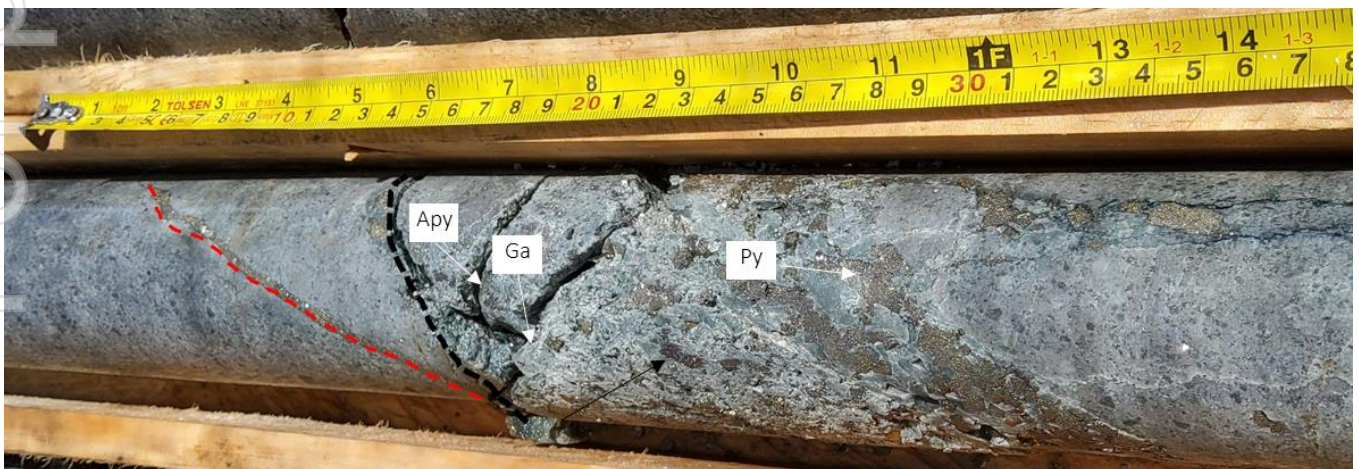
Plate 1: MGDD22-006 (35.74m). Quartz diorite with shear zone infilled by massive pyrite, sphalerite, arsenopyrite, pyrrhotite and galena, with a halo of sericite and illite-smectite.
