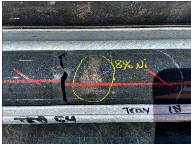
Figure 2: Example of blebby Ni-sulphide in drill core from the 12m blebby Ni-sulphide zone intersected in diamond drill hole TED54 from 159m downhole. The particular focus of the photograph is 167.5m downhole. Note that the Ni-sulphide percentage written on the core is an approximate for the individual bleb only and is from hh-pXRF spot analyses for geologists use only. Please refer to text for further details, in particular on the reliability of hh-pXRF analysis, which is also highlighted in Appendix 1.
