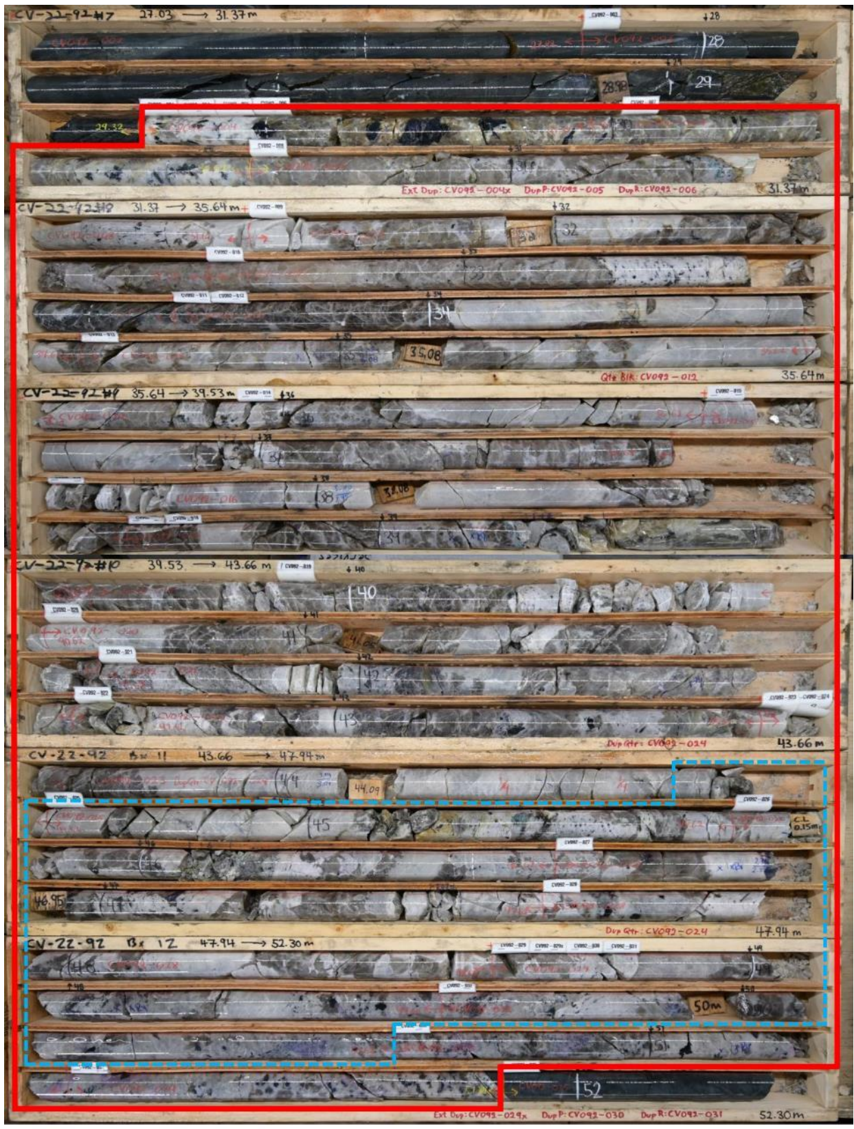
Figure 3: Spodumene drill-core intersection in drill hole CV22-092 (22.6 m at 1.56% Li 2 O, including 6.0 m at 3.19% Li 2 O)
