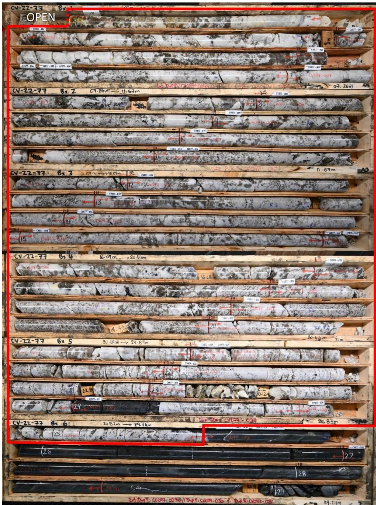
Figure 4: Spodumene drill-core intersection in drill hole CV22-077 (22.4 m at 1.28% Li 2 O), which collared in spodumene pegmatite.
